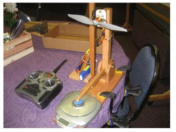
Steve showed off a device he built to measure the thrust of electric motors used in model airplanes. He operates it by remote control and he demonstrated the test platform for the members. Note the digital weight scale at the end of the lower arm. Electric motors for model airplanes? Shows just how far electric motor and battery technology has advanced.
