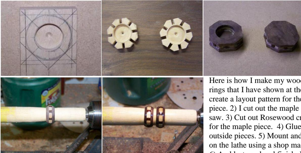
Here is how I make my wooden finger rings that I have shown at the club. 1) I create a layout pattern for the Maple piece. 2) I cut out the maple on table saw. 3) Cut out Rosewood cross inserts for the maple piece. 4) Glue on walnut outside pieces. 5) Mount and turn rings on the lathe using a shop made mandrel. 6) And last sand and finish. I used CA
