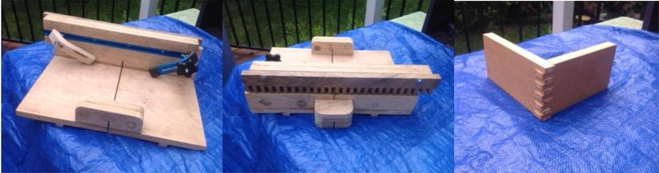
I finished making this box joint jig yesterday and tried it out this morning. It allows you to make any size box joint you want using a single, general purpose, table saw blade. The example shown in the picture is a 3/8" box joint corner. The jig is very easy to make and apparently it works fine. Keep on doing those wonderful NL's.
