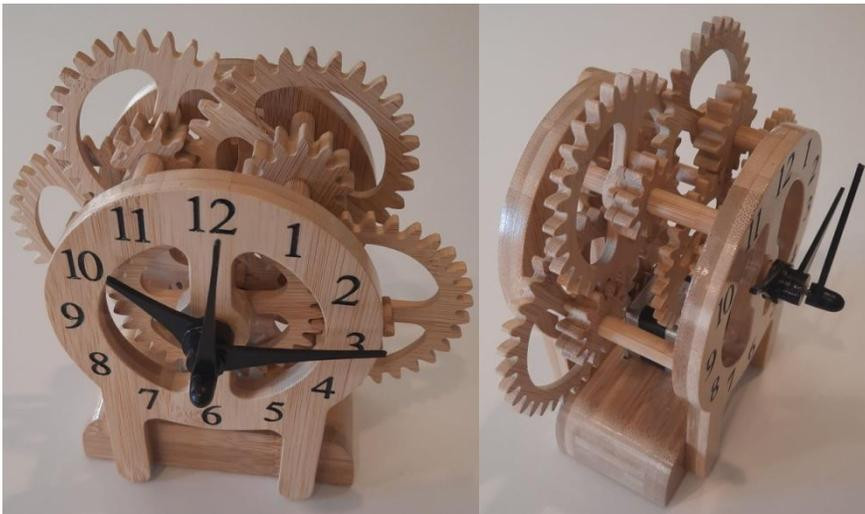
Here's my April Project Challenge entry. The clock uses an Arduino Nano processor and a custom motor driver to power a small stepper motor. The motor drives a sweep second hand with the gears providing a 60:1 ratio for the minute hand and a 12:1 ratio for the hour hand. Everything was cut on a CNC router using a 1/8" down-cut spiral bit at 60" per second. Bamboo has a nice grain pattern without showing any tendency to
