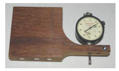
Another project shown by Mark was this jig/tool he made to simplify the setting of the knives on his joiner. It uses a Micrometer Dial Gage mounted in a block containing magnets. He locates the jig on the out-feed table near the knives. After calibrating the gage to the out-feed table he sets the gage at each knife blade and adjusts the blade to the same height as the out-feed table. I need to make one of these...
