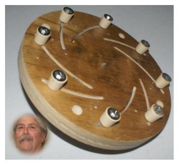
Mark brought in 2 projects this meeting. The first one on the left is his shop made Longworth chuck. This type of chuck is useful when finishing off the bottoms of turnings. The chuck mounts on his vintage lathe he recently acquired using a faceplate. He found the plans for it on the net at <a href="http://ravenview.com/blog/2010/10/17/how-to-make-a-longworth-chuck/">http://ravenview.com/blog/2010/10/17/how-to-make-a-longworth-chuck/</a>
