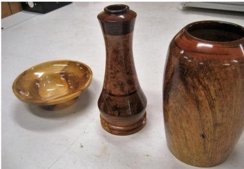
Far left: CA was used to harden soft end-grain for final turning, sanding and finishing.
