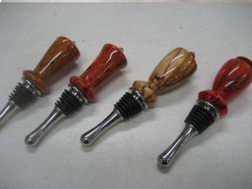
Bottle stoppers at left were made from woods that were: soft and or worm eaten. The blanks were stabilized using the heat cured plastic resin injection process. Any voids are filled. Dyes were used.
