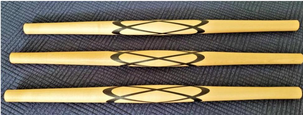
Frank ventured into the Celtic Knot world by creating these 3 Maple and Wenge French Rolling Pins. The Celtic Knot is .090 " thick and the overall dimensions are 1.2" in the center and 0.8" on the ends with a length of 18 inches.
