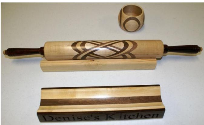
Rob took on the Celtic Knot challenge making the rolling pin and the napkin ring. The rolling pin holder was created using a parallelogram jig on the table saw. This can be a challenge as it requires many passes over the saw blade at an angle. A little sanding and you have a nice wide cove. Gee Rob, how about a demo.
