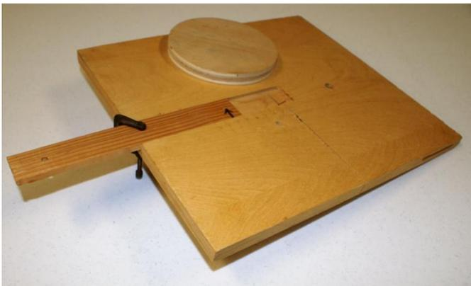
Homer showed his circle jig he uses on the band saw. He is able to set desired radiuses by sliding & clamping the slider with the circle center pin. This jig must be clamped to the band saw table with the blade gullet even with the center pin.
