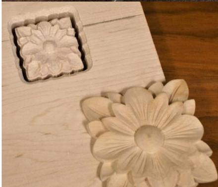
A program (application) on the computer controls the scanner and stores the digitized 3D data image (the pattern) of the target item. Using the computer John is able to touch up the scanned image, resize it and basically modify the pattern to meet his needs. Once he is happy with the pattern he can send it to his CNC machine to be reproduced.
