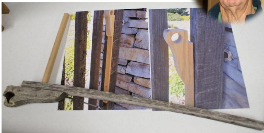
Homer brought in an interesting item. It is an old "gate latch" made of Oak that no longer works well. He made a new one mounted to the gate in the picture. The dowel is held in place by the spring action of the Oak stick. The stick has enough spring to allow the dowel to be pulled back releasing the gate. The old one lasted 20 years!
